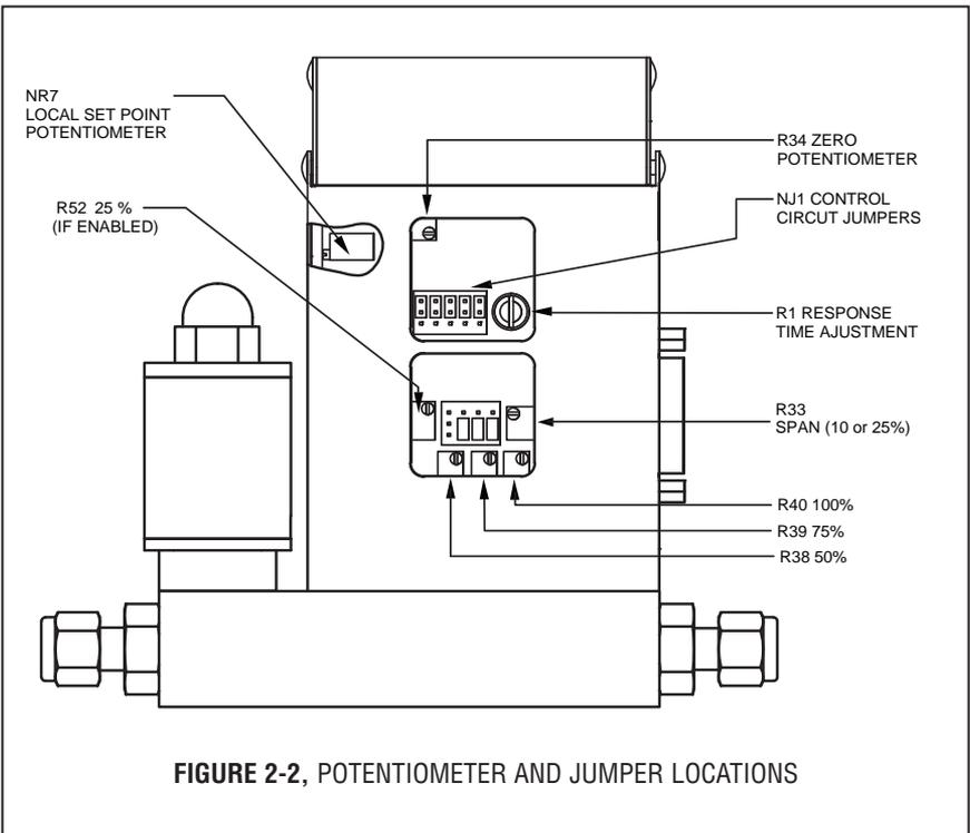
FIGURE 2-2, POTENTIOMETER AND JUMPER LOCATIONS
