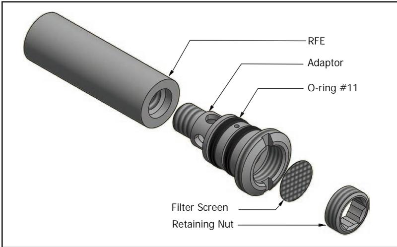
5. Clean or replace each of the removed parts as necessary. If alcohol is used for cleaning, allow time for drying.
