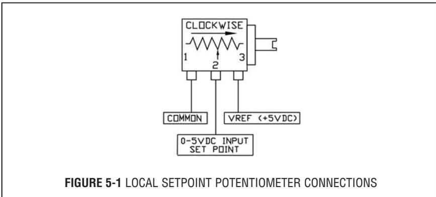
**FIGURE 5-1** LOCAL SETPOINT POTENTIOMETER CONNECTIONS
