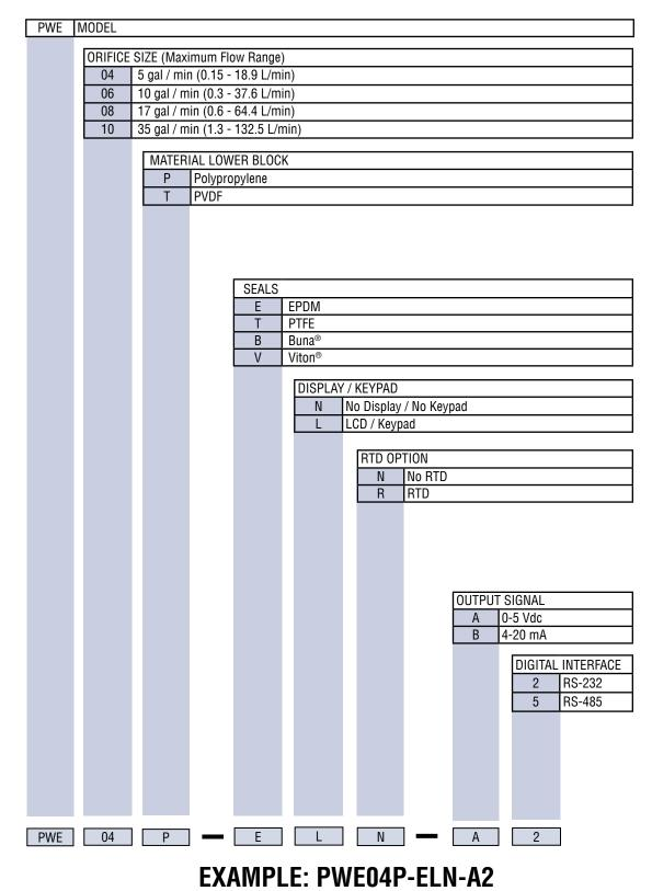
Digital Paddle Wheel Meter, Maximum Flow 5 Gal. per minute, Polypropylene Lower Block, EPDM Seals, LCD Keypad, No RTD, 0-5 Output Signal with RS-232 Digital Interface.
