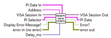
Reads the instrument's Process Information parameters: Mass Flow Rate, Totalizer reading and Flow Alarm status and composes the cluster of string representing following parameters: Mass Flow Rate (MEU), Totalizer value (MEU), Flow Alarm Status [N,H,L] and Diagnostic Register value.
