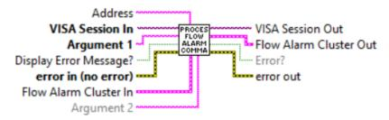
Reads and writes Flow Alarm parameters. Refer to ASCII commands set in the XFM operating manual for proper values of the strings wired to the Argument#1 and Argument#2 inputs. This Sub-VI parsing output data frame and updates corresponding parameters of the Flow Alarm cluster.
