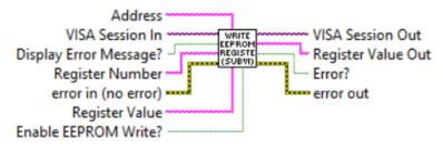
Writes specified value to the to the instruments corresponding EEPROM register. Returns response as a string (unedited) which represent EEPROM register value.
