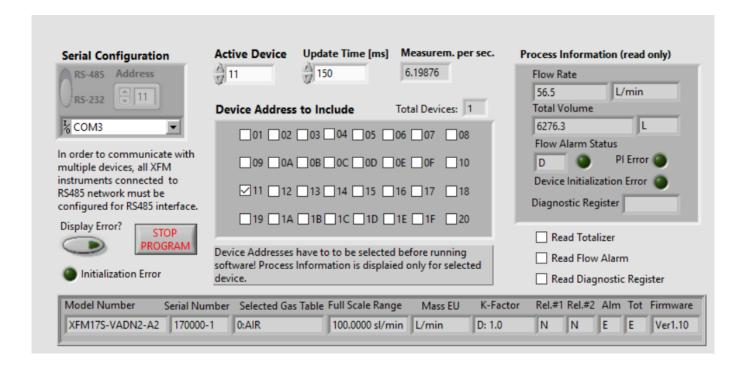
Simple example program initializing the COM port, determining the instruments configuration data for up to 32 XFM instruments, (configuration data will be collected only for instrument addresses which are selected in the "Device Address to Include" control cluster), acquiring the data of the same number of instruments, displaying the data only for the one with the selected "Active Device" address.
