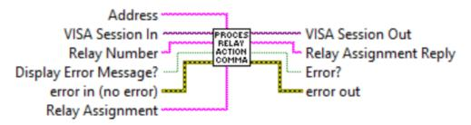
Reads and writes instrument's Relays assignment parameter. Refer to XFM ASCII commands set (Paragraph 8.3 in the XFM operating manual) to determine valid values for "Relay Number" and "Relay Assignment" input terminals.
