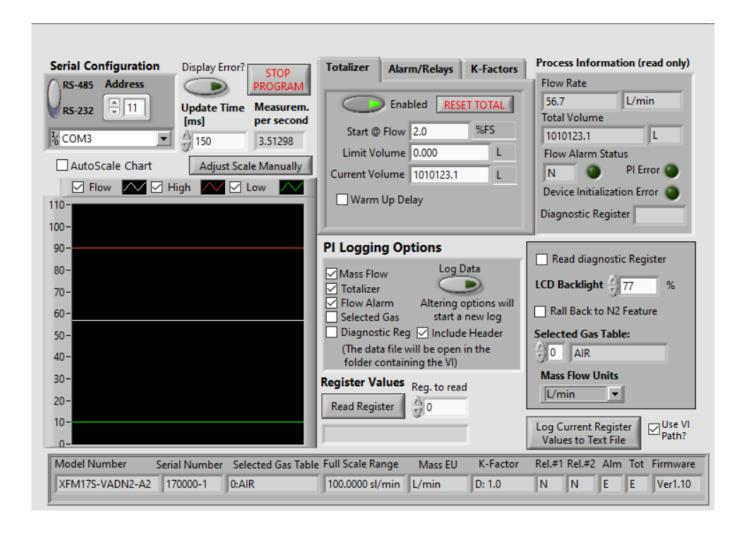
This example program utilizes almost all VI's included in the AALBORG XFM LabView Driver Library. In addition to the simple program example it provides access to the PI data Waveform Chart, Totalizer, Alarm, Relay Assignment, K-Factor, Diagnostic Events and Process Information data logging settings and features of the XFM instruments. It also allow to change active Gas Table, select desired Mass Flow units of measure and read instrument's EEPROM registers.
