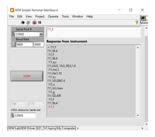
Example VI for communicating with AALBORG XFM instruments via serial communication interface using ASCII commands set (see XFM instrument operating manual for complete list of supported commands). For RS485 interface the start character is always! and two characters of address with coma delimiter in the end must be submitted before each command (see example below). !11.F
